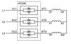
The motor connection depends on the supply voltage, which in this example is a star connection.
