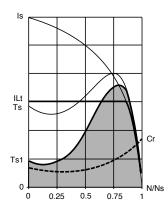
Curves Ts and Is represent the direct line starting of an asynchronous motor.
