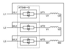
Connection in the motor delta winding
