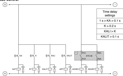
BPMn: "Run" button motor n BPAn: "Stop" button motor n R1 must be configured as an isolating relay (r1 = r1l)
