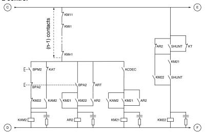
BPM1: "Run" button motor 1 BPM2: "Run" button motor 2 BPA1: "Stop" button motor 1 BPA2: "Stop" button motor 2
