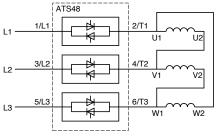
The motor connection depends on the supply voltage, which in this example is a delta connection.
