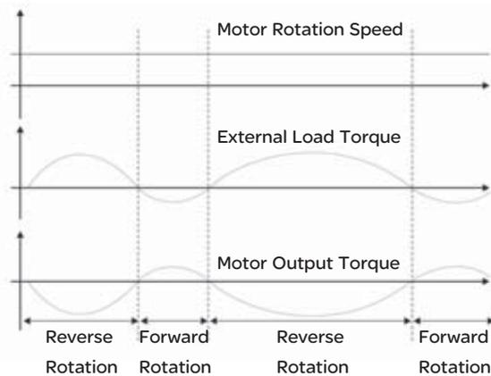
External load torque in reverse direction:  $T_L \times \omega_r$   $T_L$  : External load torque
