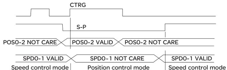
Figure 1. : Speed / Position Control Mode Selection
