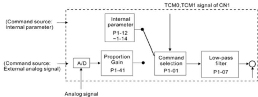
The command source is selected according to the state of TCM0, TCM1 and parameter P1-01 (T or Tz).
