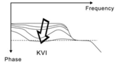
STEP 3: Select the value of KVI, if the value of phase margin is too small, re-adjust the value of KVP again to obtain the value, 45deg of phase margin.
