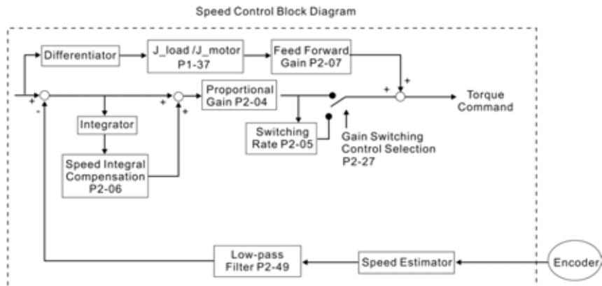
5: AutoMode (PDFF) [Fix the ratio of Load Inertia to servo motor inertia and response level can be adjusted]
