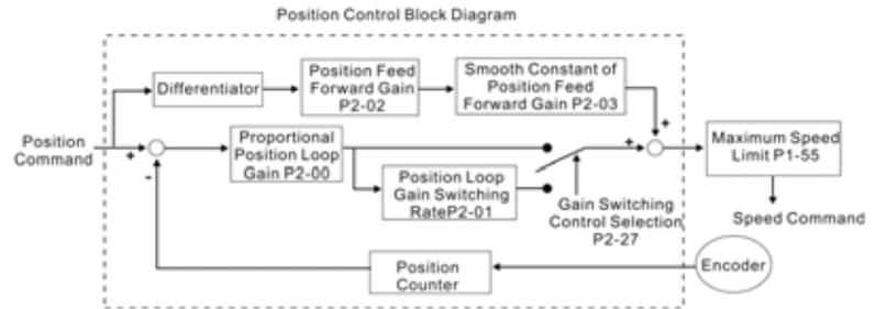
When the value of Proportional Position Loop Gain, KPP is too great, the position loop responsiveness will be increased and it will result in small phase margin. If this happens, the rotor of motor will oscillate.
