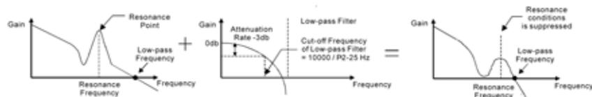
When the low-pass filter (parameter P2-25) is adjusted from 0 to high value, the value of Low-pass frequency will become smaller (see the figure on page 6-26). The resonant condition is improved but the frequency response and phase margin will also decrease and the system may become unstable.
