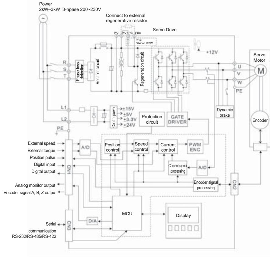
**Figure 3.7 Basic Wiring Schematic of 4.5kW and above models**
