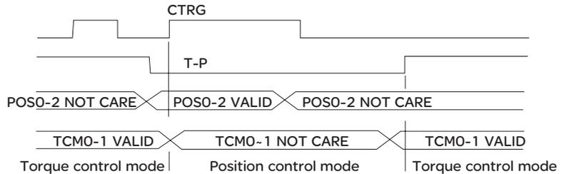
Figure 3. : Torque / Position Control Mode Selection
